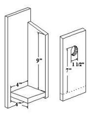
Extend the back wall panel beyond both top and bottom. Drill pilot holes in these long panels for mounting. Drill an extra mounting hole inside the box just under the roof. Stagger these holes so that all are not in line along a single wood grain. Holes in line with grain can weaken and cause wood to split.
